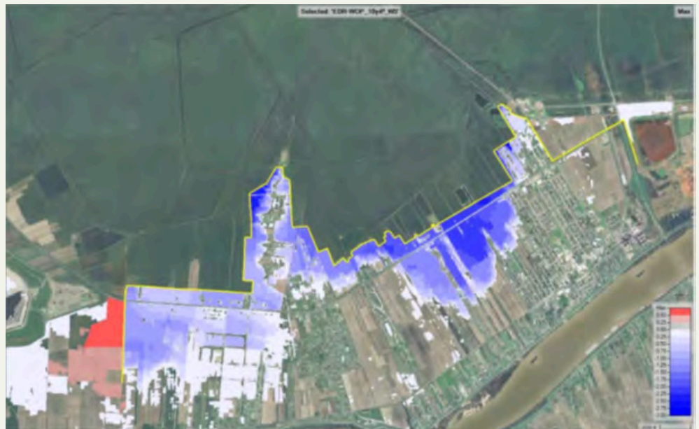
Maximum Depth With-Project Conditions minus Without- Project Conditions for the 10- year Precipitation plus 100- year Surge Event, EDR/GRR Levee Alignment
